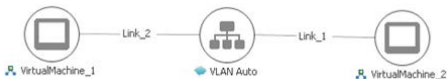
Figure 28. Two VMs Connected to a VLAN
